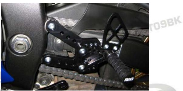
Connect the original gear shaft adaptor with the R&G Gear shaft and connect the shift lever to the original gear lever position.
